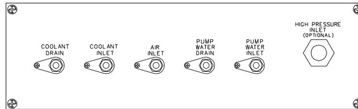
**Air Inlet, Pump Water Drain/Inlet**
