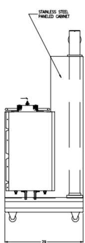
100 PSI AIR SUPPLY WATER OUTLET, 1/4 FPT DRAIN, FACILITIES RECD. WATER INLET, 1/4 FPT. 30 PSI SUPPLY REQUIRED.
