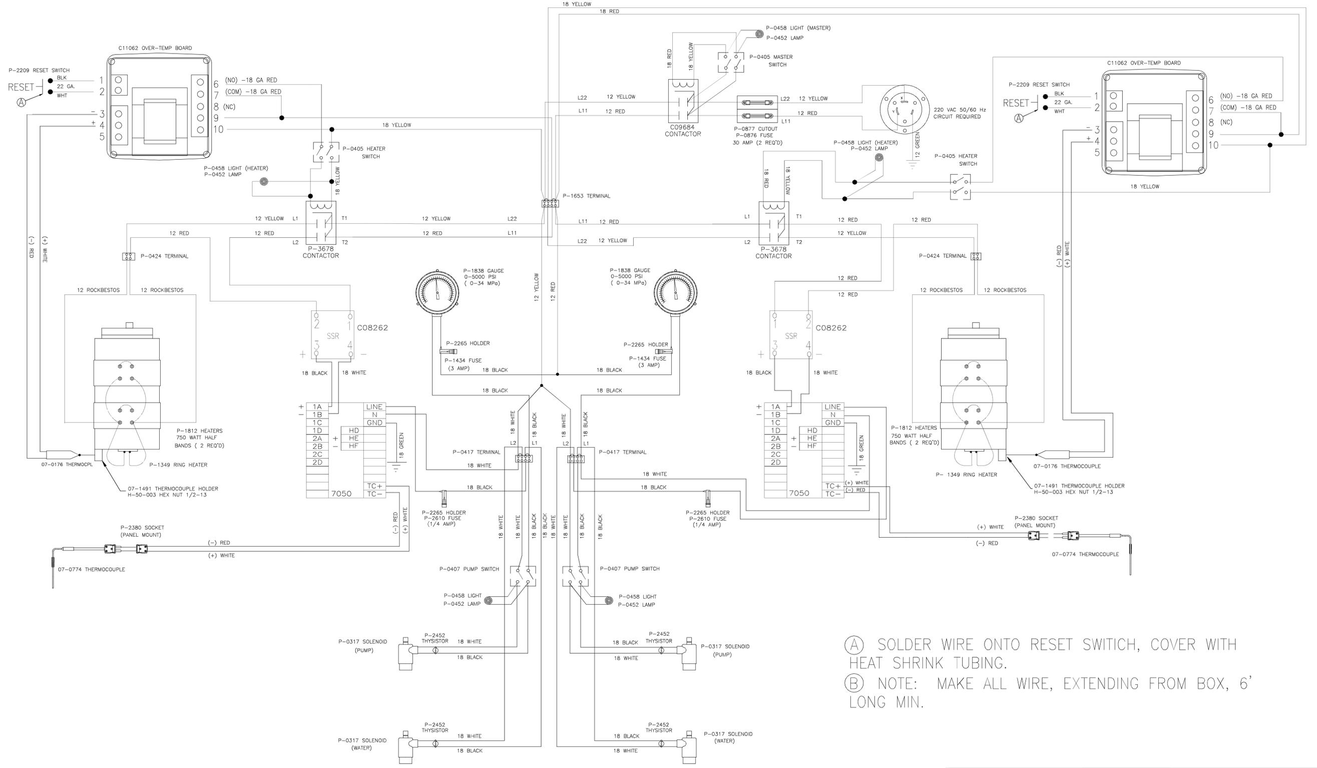
Ⓐ SOLDER WIRE ONTO RESET SWITCH, COVER WITH HEAT SHRINK TUBING.
