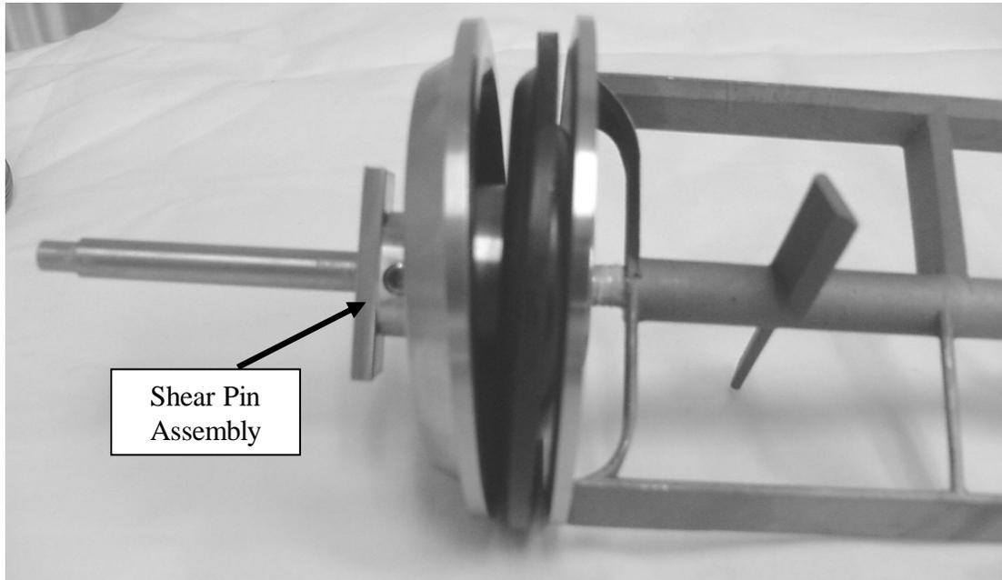
4. Install the complete paddle assembly into the slurry cup.
